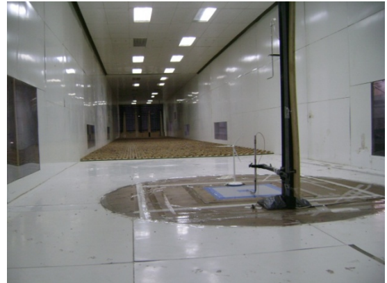
Figure 2. Wind turbine model and measurement device in the test section
