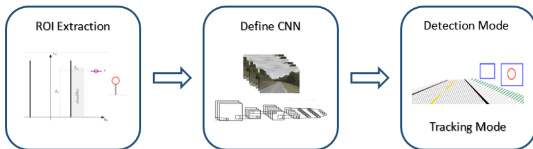
Figure 4.1 Diagram illustrating the process for the recognition of traffic signals.
