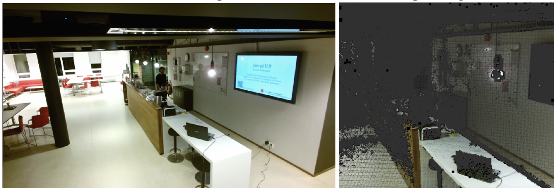
Figure 7.4: Image of a subject walking far away from the camera in the back of the room. Both cameras are capturing the scene. On the left, we see the RGB image and the subject walking in the back of the room. In the image on the right, we can identify the issue the IR camera is not able to detect the person since he is out of the depth range.
