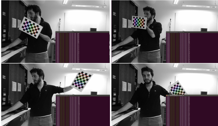
Figure 3.1: Chessboard being capture in different angles and recording different patterns to update the camera matrix and the distortion coefficient matrix.
