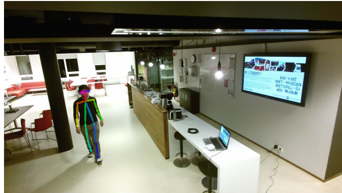
Figure 2.1: Example of Openpose being used in one of the experiments. It is possible to see that openpose can successfully recognize the human skeleton. The image resolution is 960x540.
