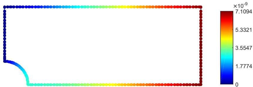
(a)  $u_1$  - MEC.
