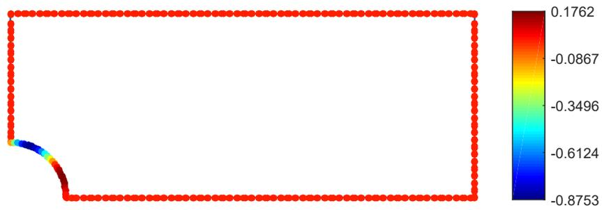
(a)  $\sigma_{12}$  - MEC.
