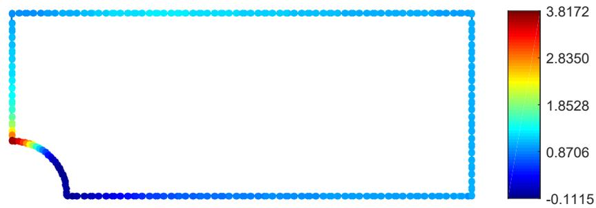
(a)  $\sigma_{11}$  - MEC.
