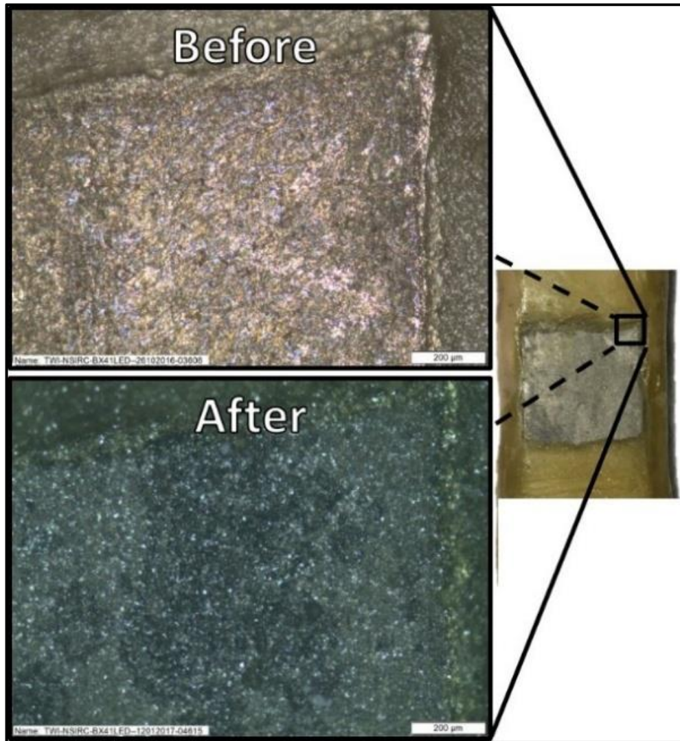
Figure 75: Comparison of the corrosion surface of the working electrodes before and after the test. Test conditions: V/S of 0.2 ml/cm 2 , 3.5%wt. NaCl brine, FR/SS of 0.0785 ml.min -1 cm -2 , 1 atm of CO 2 and 30±2 °C.
