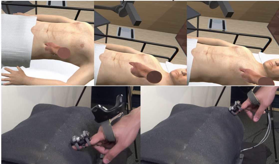
Figure 3.24: Palpation example using our methodology to render softness in a medical application: User is touching a soft part and then moving to a hard part: the device releases at different rates to render the different parts of the body.
