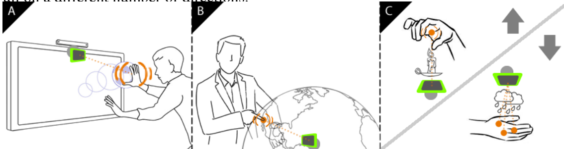
Figure 3.3: Example of different applications where the ULTRAMOTION device. (A) The device can follow the user's hands to provide directional feedback and even in other body parts for attentional redirection; (B) User can interact with big volumes and holographic visualizations; (C) ULTRAMOTION can also allow Ultrahaptics to deliver stimuli on a different number of directions.
