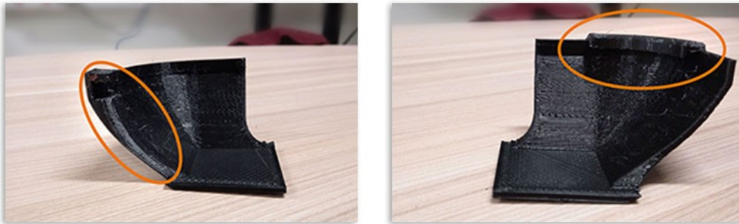
Figure 3.7: Details of the security grabs placed in the holder
