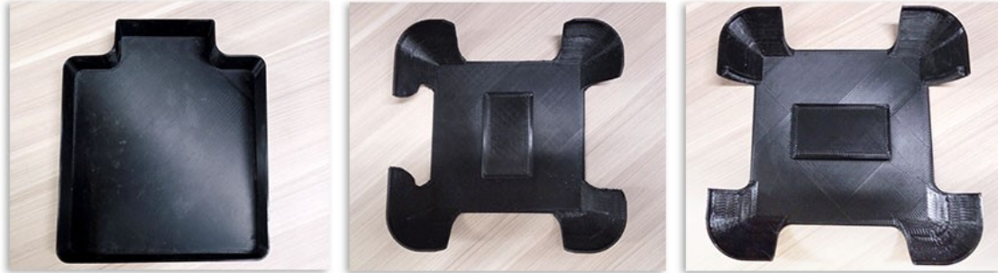
Figure 3.6: Different alternatives for the 3D printed piece made for holding the Ultrahaptics device: Left: early prototype used to verify dimensions, Center: Second model with a more robust composition and less material. Right: Third model with lateral supports and grabs in the bottom corners
