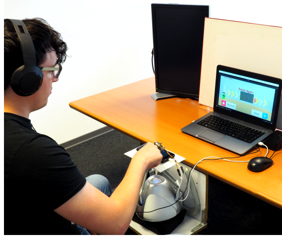
Figure 3.19: Friction setup: Subjects sits down in front of the setup and performs the swiping looking at the screen.
