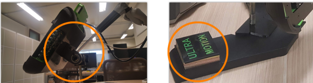
Figure 3.8: The manipulations are done through the level (left). An extra weight keep the ULTRAMOTION from drifting (right) during manipulation.
