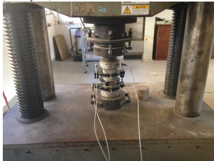
Figure 1. Press and sensors for the measurement of dimension variations.
