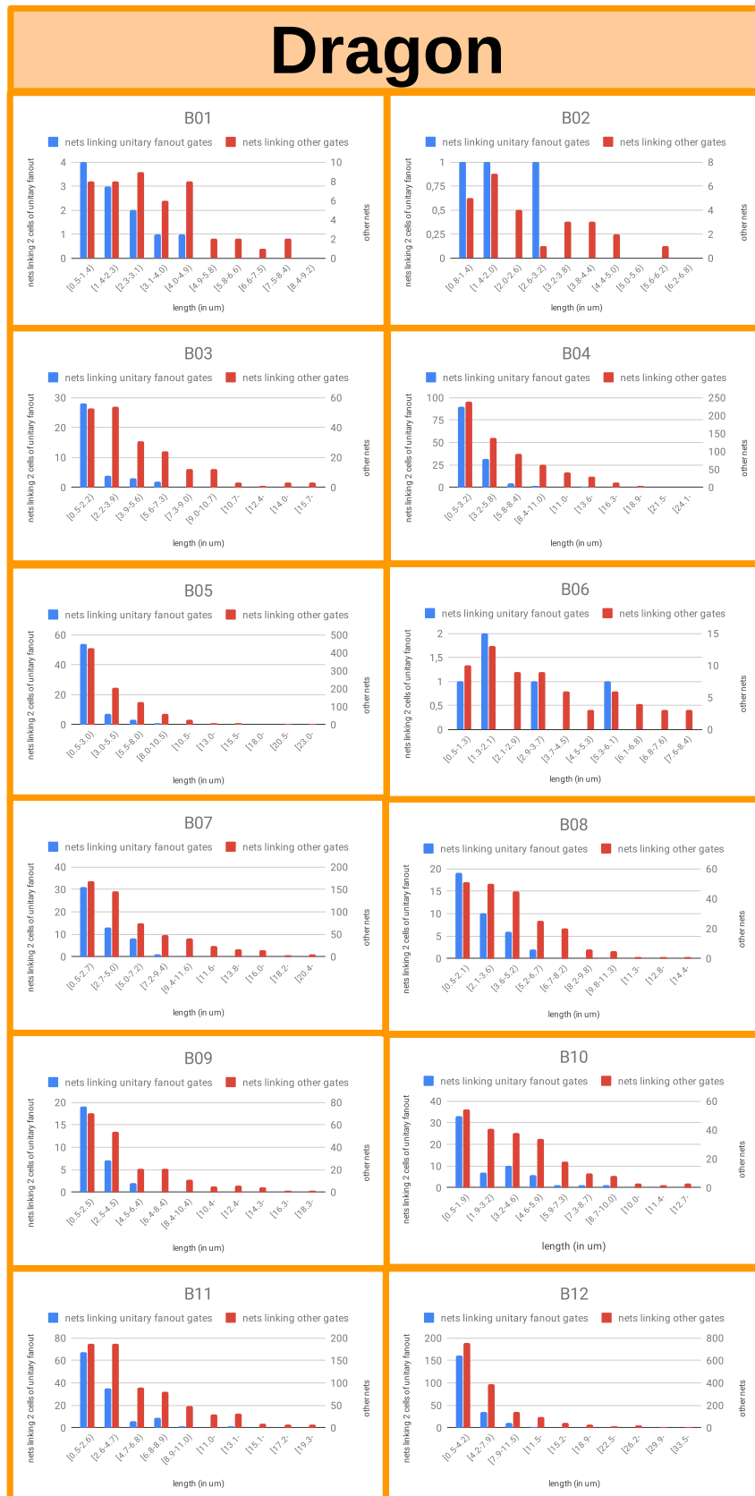
Figure 5.3: Plot of the distribution of net length estimation divided into nets linking two unitary fanout cells and other nets from circuit B01 to B12, according to Dragon placer.
