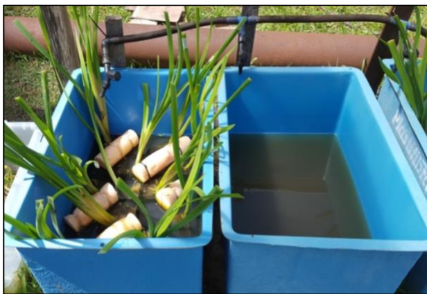
Fig. 3. Floating structure with polyethylene floating buoys supporting ten macrophytes with a Control tank aside. Mesocosm floating wetland system filled with the raw wastewater from the Water Quality Recovery Station of university campus (UFRGS).
