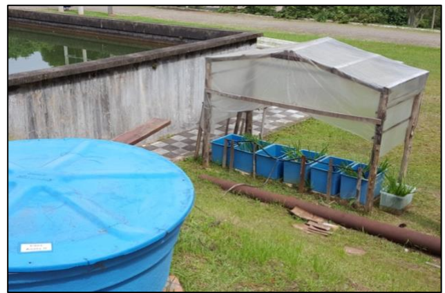
Fig. 4. The six tanks (Macrophytes and Controls) were protected from the rain to avoid wastewater dilution with a transparent material that allowed sunlight to reach the macrophytes used in the mesocosm floating wetland system.
