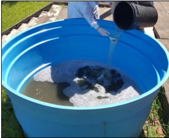
Fig. 1. A tank with 1000 L capacity was used to homogenize the raw wastewater collected from the Water Quality Recovery Station of university campus (UFRGS). A small sieve was used to remove sticks and leaves.
