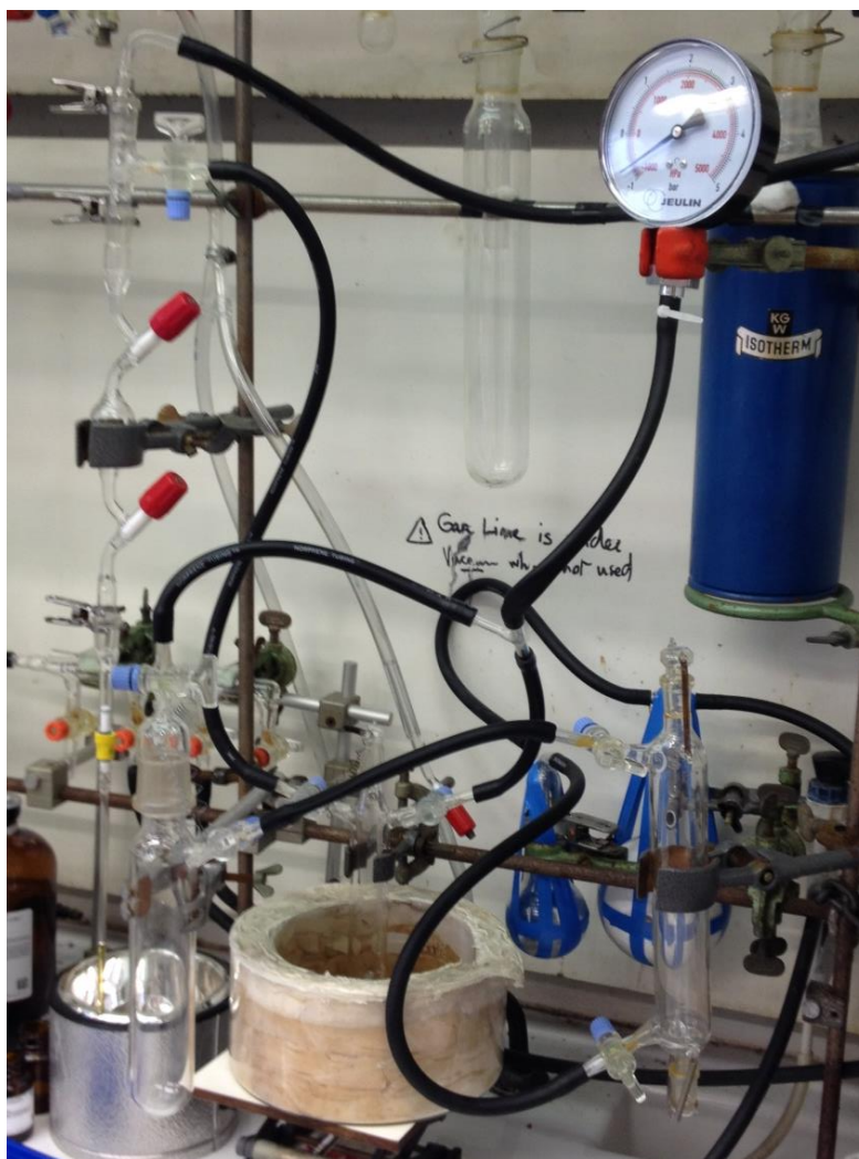
Figure S1. CO 2 injection system
