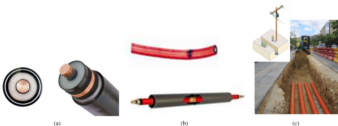
Figure 1. Underground high-voltage cables: (a) cross-section of typical cables; (b) Common pathologies in the cables; (c) Typical installation.
