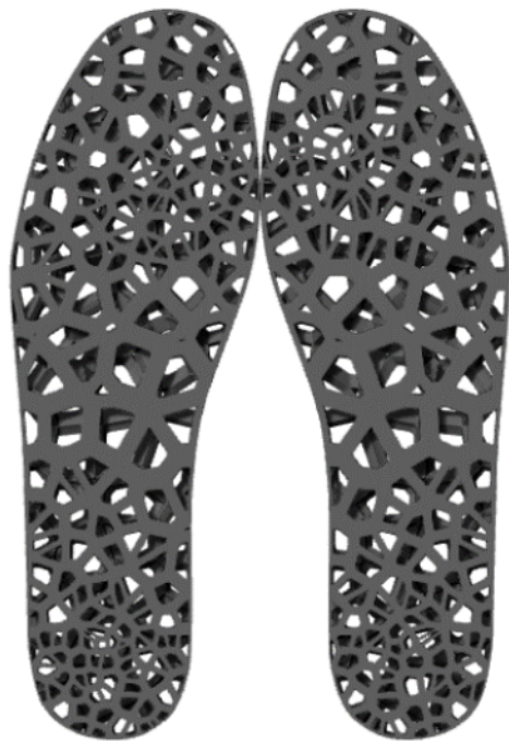
Figure 9 Top profile of baked meshes, independent cell pattern for left and right midsoles.
