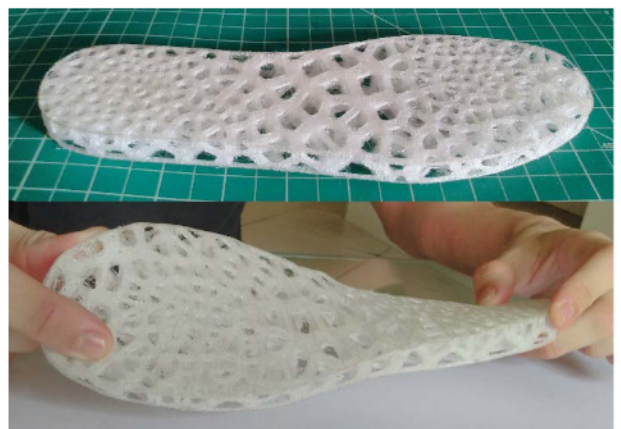
Figure 12 Pictures of 3D printing final geometry in white-translucid and flexible TPU.
