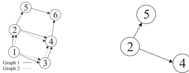
Figure 8 – Graph IDs and neighbors configured in node 2 for a given Graph ID.
