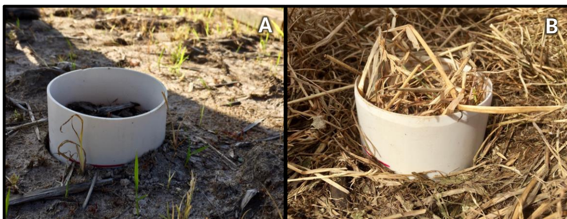
Figure 18. Collection of undisturbed samples with PVC tubes in the traditional rice system (A), and integrated crop-livestock system (B), prior to rice sowing (October 2018), to conduct the greenhouse experiment using ^{15}\text{N} -labelled fertilizer.
