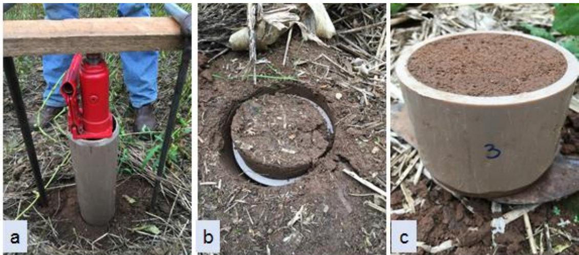
Figure 18. Sampling of the large samples using a hydraulic bottle jack (a), soil core in 4 cm below to the surface (b), and soil core after knife-trimming.
