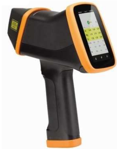
Figure 41: Typical handheld operation LIBS sensor (adapted from RANULFI et al., 2018)
