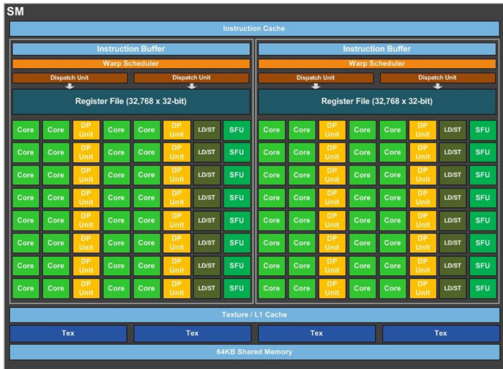
Figure 1 – Pascal Streaming Multiprocessor of the GP100 chip
