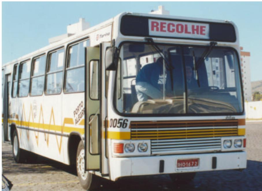
FIGURA 4.2 – Ônibus Mercedes – chassi normal.
