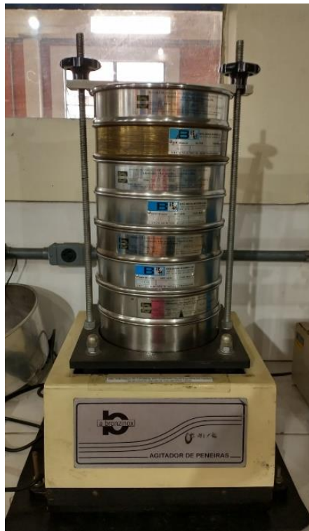
Figure 3.2 – Sieves assembled in the sieve shaker.
