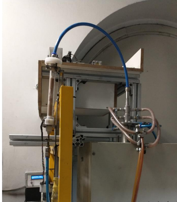
Figure 3.7 – Feeding system connected to the fuel injector at the top of the DTF.
