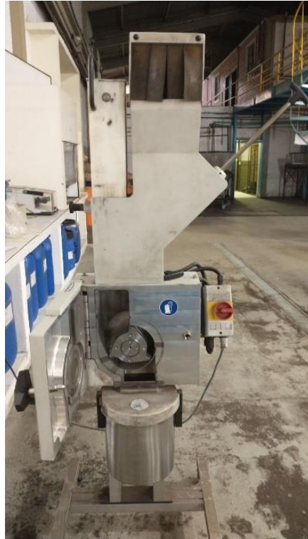
Figure 3.3 – Cutting mill SM 100 from RETSCH.
