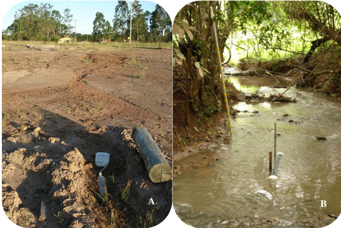
Fig. 3. A – Sampler 1, installed on the soil surface of contaminated area. B – Sampler 2, placed inside of water body that crosses the contaminated site.
