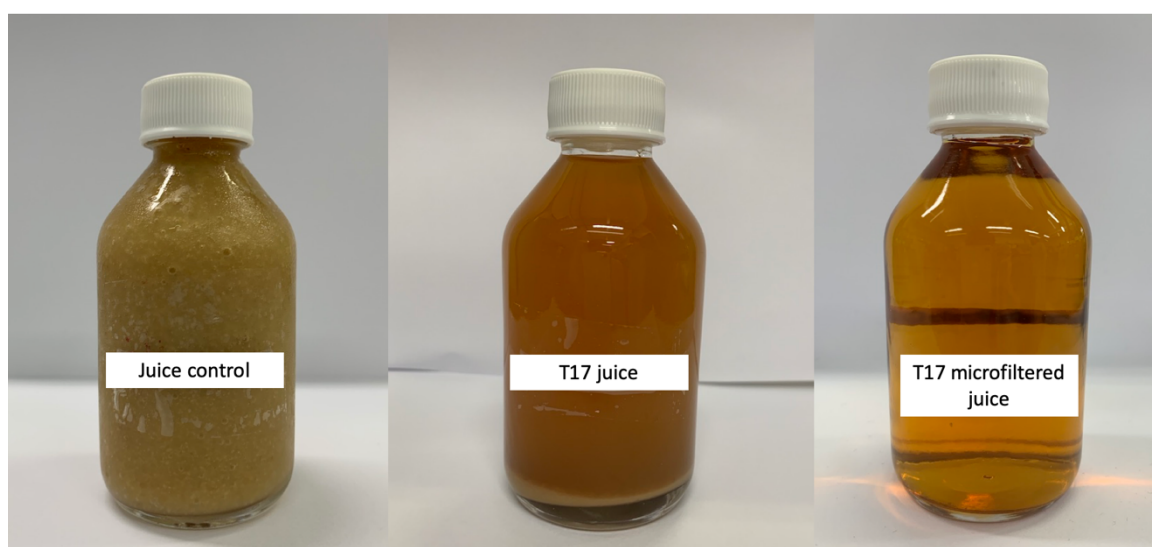
Figure 3. Three feijoa juices - juice control: raw; T17 juice: treated with Pectinex enzyme ( 10 \text{ U.mL}^{-1} and 5 \text{ U.mL}^{-1} ) and pasteurized; and T17 microfiltered juice: with addition of the microfiltration process.
