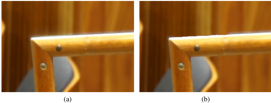
Figure 6.11: Light aura around handrail due to misplaced depth values. (a) Aura is present due to wrong depth values. (b) After fixing some depth values on the top-left border of the handrail, the aura is absent on that region, but still present on the other regions.
