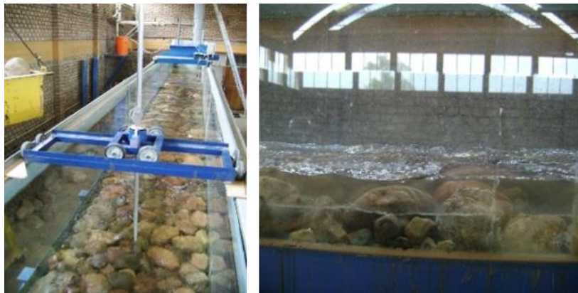
Figure 1.- Tilting flume with artificial large-scale roughness bed. Limnimeter and laser profile depicted on left figure
