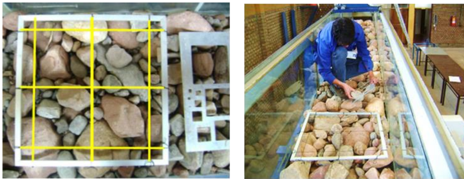
Figure 3.- Metallic frame (0.60 m \times 0.60 m) and gravelometer (left) used for the sampling method of Bunte & Abt (2001) (right)
