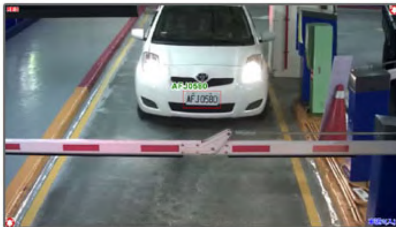
Figure 1.1 – Example of ALPR system available in the market with restrictions related to the object position for LP recognition.
