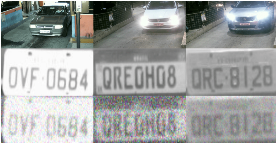
Figure 4.3 – RodoSol image examples used as high and low resolution pairs to fine-tune TSRN.
