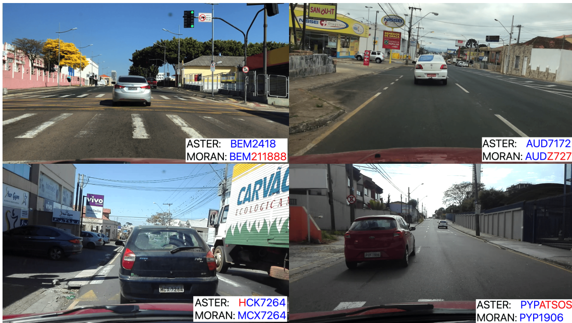
Figure 5.2 – Result samples from experiments 1 and 2 using ASTER and MORAN in the OCR module.
