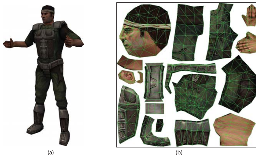
Figure 1.1: Texture mapping. Item (a) illustrates a 3-D triangular mesh. We can see on (b) the mapping of the mesh over a texture. Based on this mapping it's possible to define a color for each point on the 3-D mesh surface as the color mapped in parametric space.
