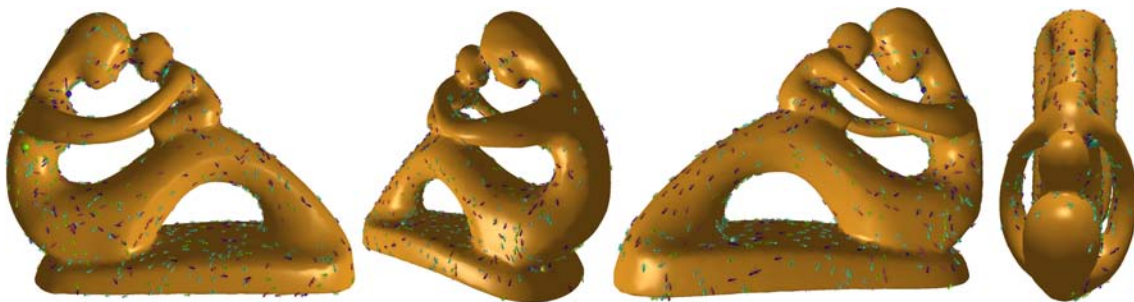
Figure 6.1: Four different views of a scene where agents navigate on the surface of a complex triangular mesh. Agents are color-coded by their different objectives. The system supports path planning of multiple agents on non-planar surfaces, and imposes no limitation on the domain mesh, such as this mesh with more than one genus.
