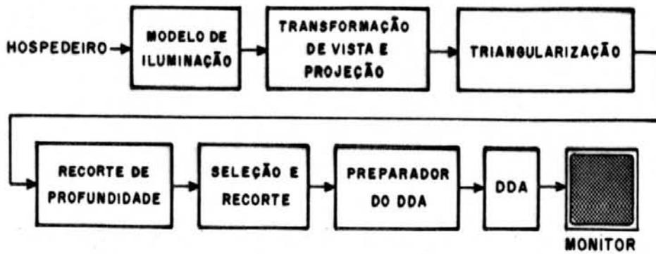
fig. 4.33 - Pipeline do GIRD
