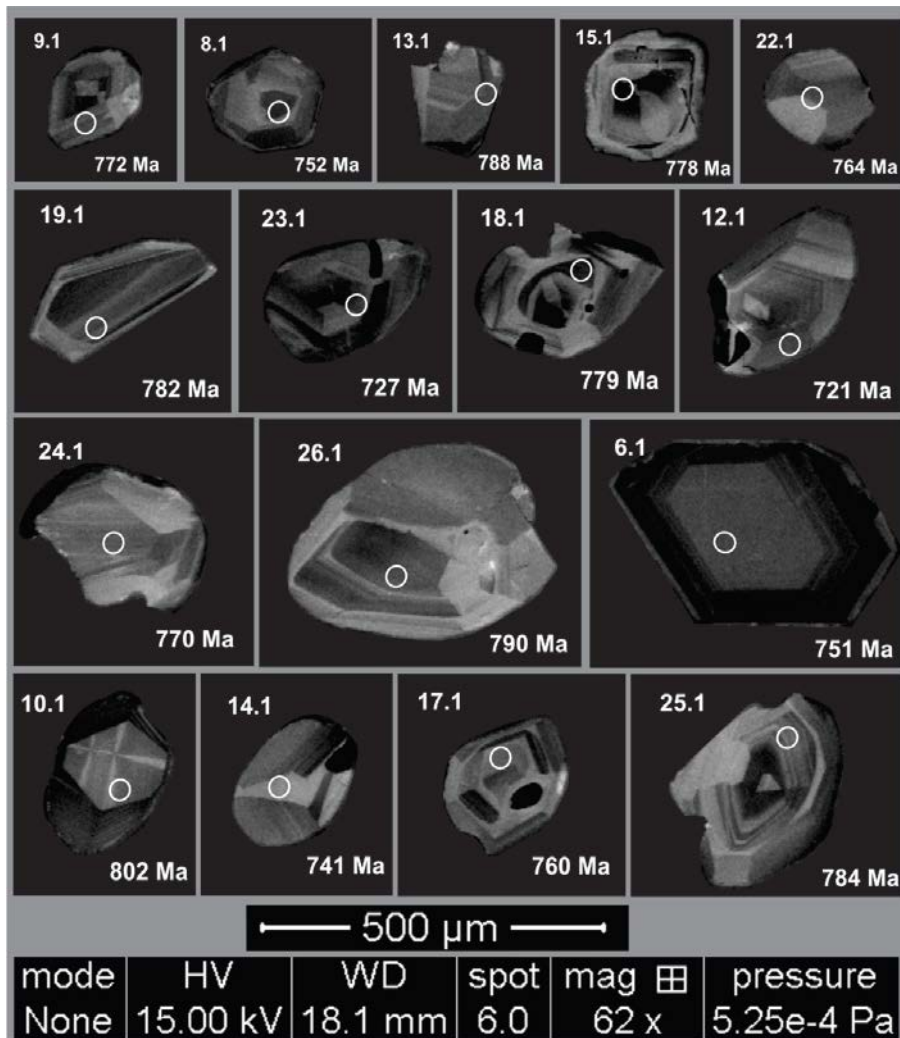
Figure 9 - Cathodoluminescence image of zircon grains analyzed from meta-agglomerate BOS-3 showing the spot locations and the corresponding ^{238}\text{U}/^{206}\text{Pb} ages.
