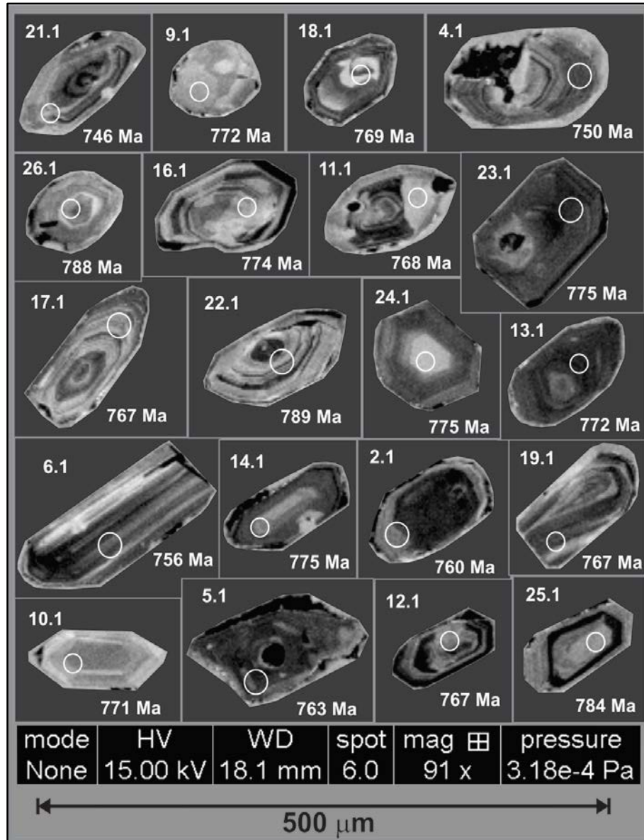
Figure 7 - Cathodoluminescence (CL) image of zircon grains from metacrystal tuff BOS-2, showing the location of spot analyses and the corresponding ^{238}\text{U}/^{206}\text{Pb} ages.
