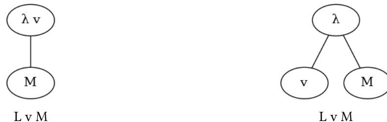
Figure 5.2: Difference between implicitly putting the variable of the abstraction in the node, and explicitly putting the variable as a leaf, as implemented in this work.
