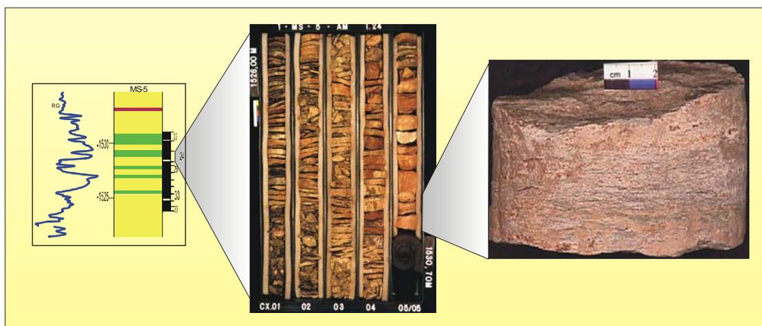
Fig. 6.8 – Litofácies A5: Arenito com “climbing-ripples”.
