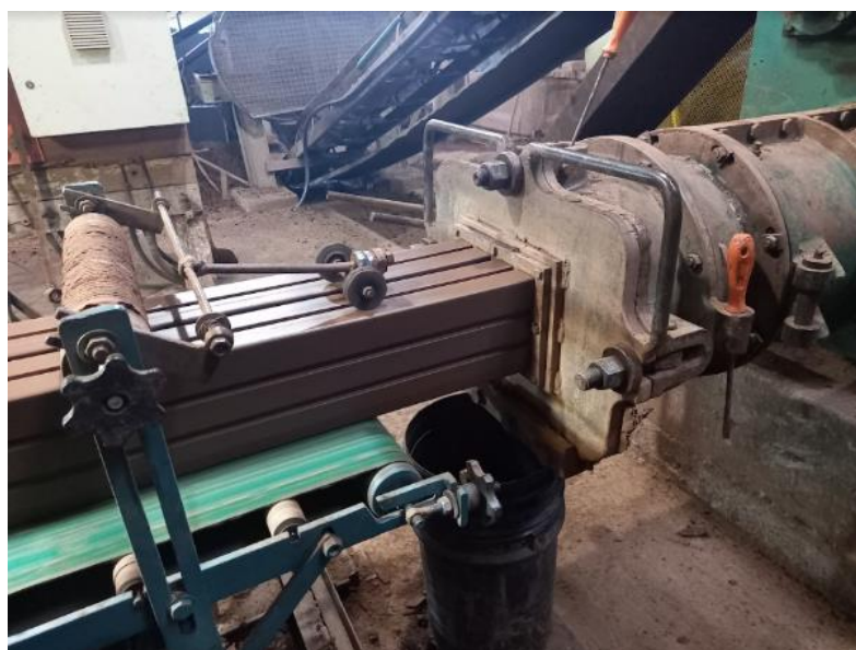
Figure 3: The appearance of industrial-made brick with 20% waste glass extruded in the brick plant.
