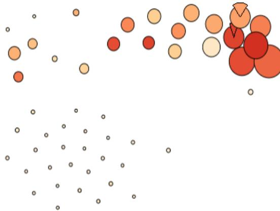
What Figure 4.19 accomplishes is quite interesting. In a small space, we've encoded 4 different aspects of the data: similarity (position), class size (glyph radius), change in class size (delta pie slice size), and average cyclomatic complexity value for each class's methods (color). And best of all, without any clutter or misinformation.
