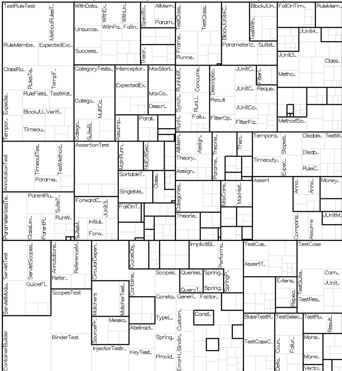
Classes might change in size from one revision to the next, yet Squarified Treemaps are inherently static, therefore in order to add information about the dynamic LOC metric value without rearranging the layout, we have encoded in the filled rectangle area the current metric value. The increasing/decreasing of value is shown with a smooth transition between states.
