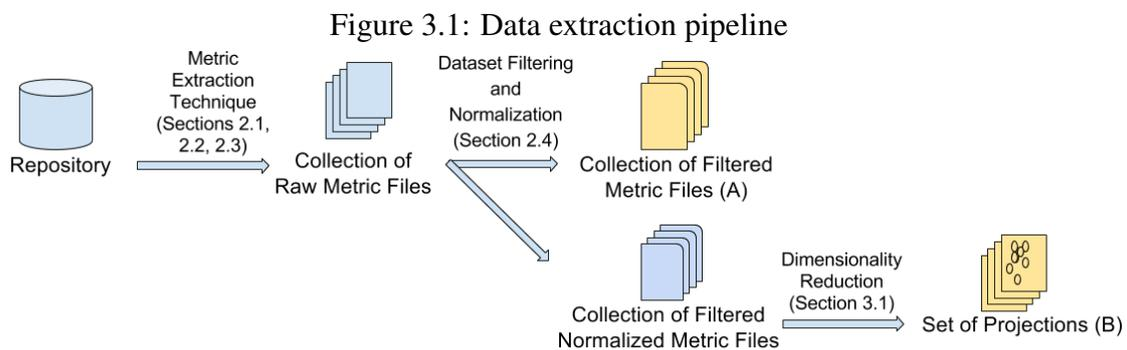
Figure 3.1 illustrates the pipeline that takes a software repository and outputs the two datasets (A and B) that are used in our visualization tool.
