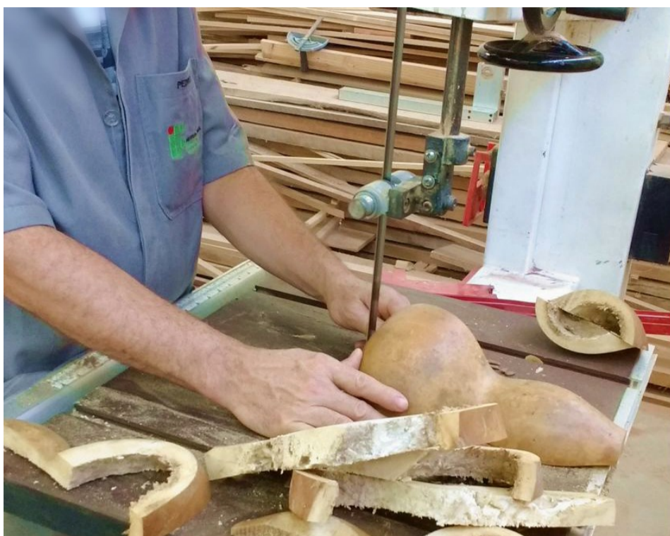
Longitudinal cutting process of the pieces, carried out in equipment called band saw (Photo: Danieli Nejeliski/disclosure)
