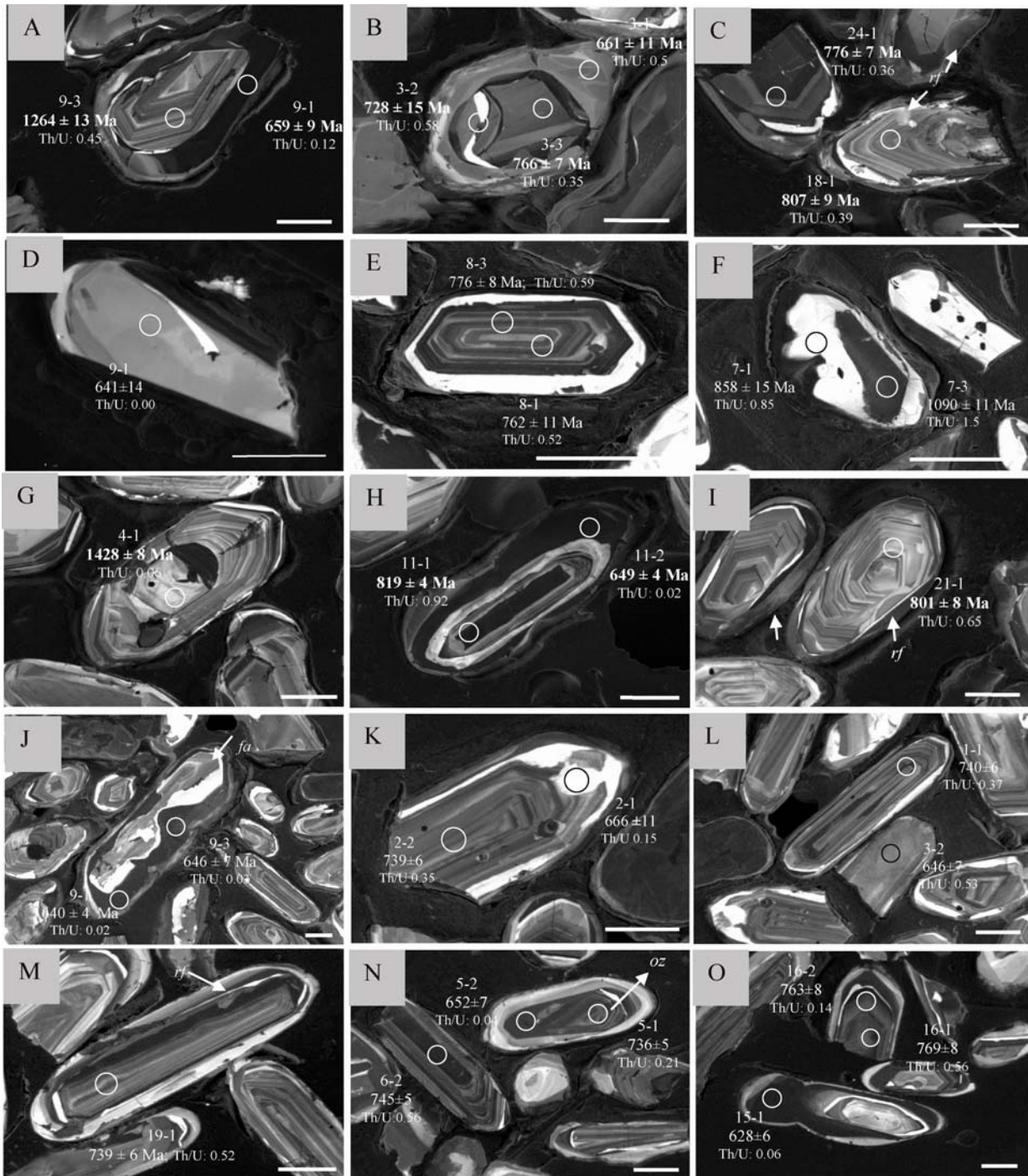
Figure 4: Cathodoluminescence images of zircons from the mafic granulites and gneisses. Figure A, B and C: sample AC-133-B; Figure D, E and F: sample UY-2-A; Figure G, H and I: sample AC-296-M; Figure J, K and L: sample AC-373-B; Figure M, N and O: sample PCH-0869. The scale bars are 50 \mu\text{m} . Abbreviations: rf : recrystallization fronts; fa : faded areas, oz : oscillatory zoning.
