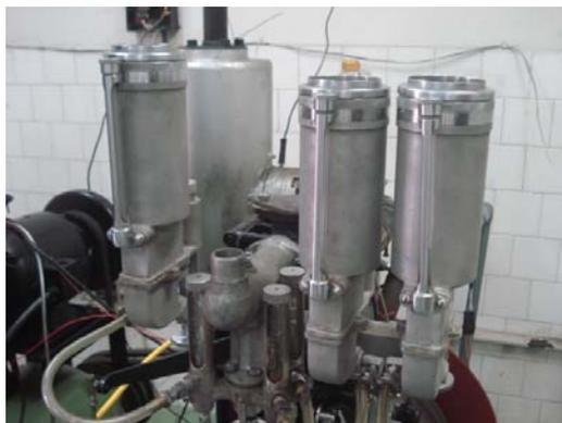
Figura 3.2 – Carburador do motor ASTM CFR.
