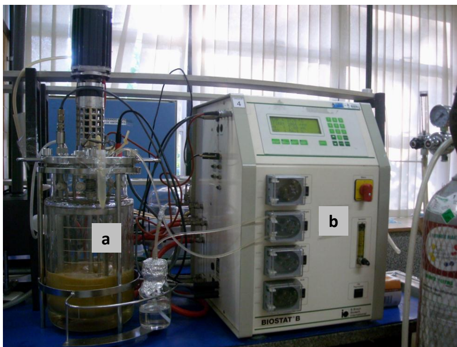
Figura 3.1 Biorreator Biostat B (B. Braun Biotech International) (a) vaso do biorreator (b) unidade de controle do biorreator
