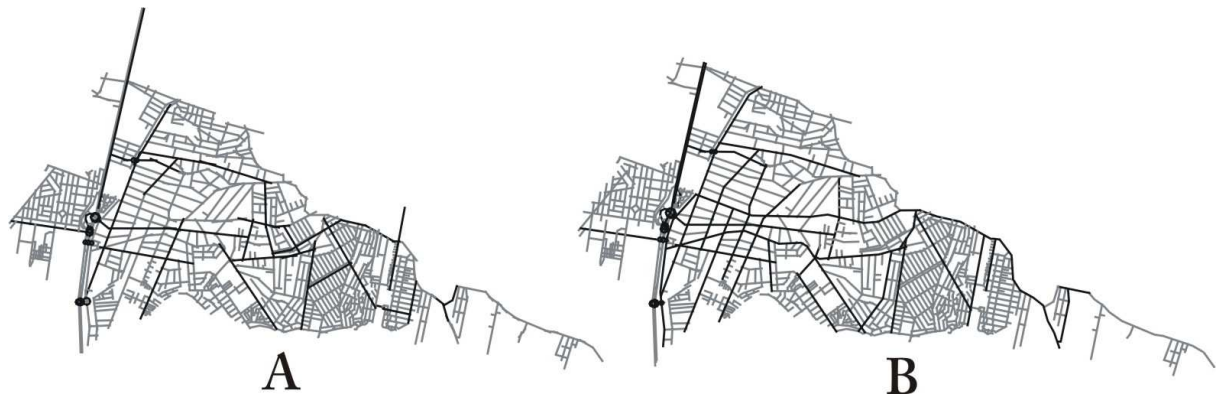
Figure 3 Choice model processed in axial lines map (A) and continuity lines map (B) - Esteio
