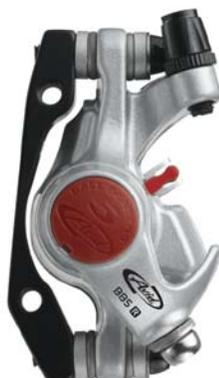
**Figura 118 – Caliper de freio a disco Avid BB5 Road**
