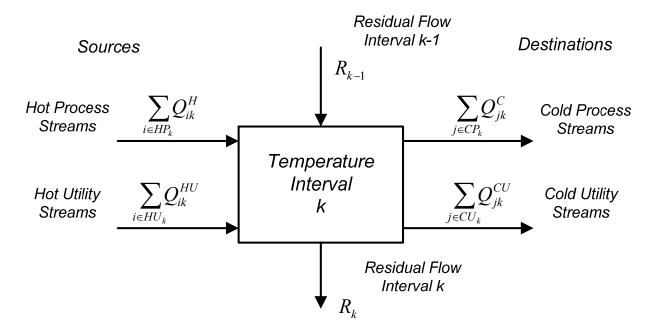
**Figure 3.5:** Heat Flow pattern of *k-th* temperature interval.
