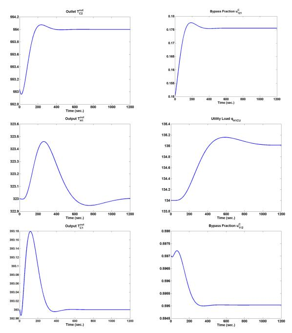
**Figure 7.16:** Servo response for control loop 4, and effect on loop 1 and 3.
