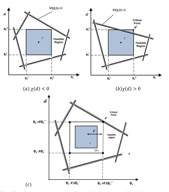
Figure 7.A: Geometric interpretation of Feasibility Test (a,b) and Flexibility Index (c).
