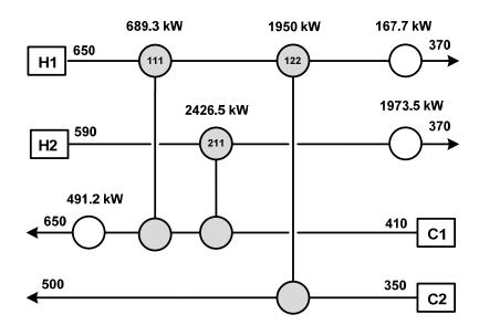
**Figure 5.5:** Nominal Configuration for Example 1.
