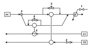
Fig. 1. Possible manipulated inputs in HENs.
