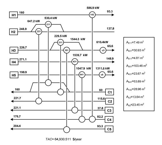
**Figure 4.5:** Heat Exchanger Network for Example 3 from the MINLP solution.
