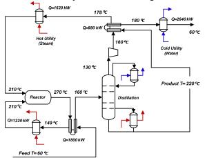
Fig. 2. Simple process with reaction, separation and heat exchangers.
