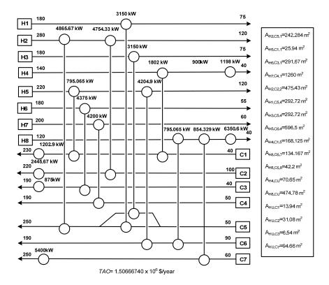
**Figure 3A.8:** HEN Configuration for the Case Study 03 using Synheat.
