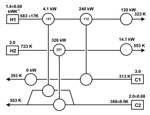
**Figure 6.5:** Final Configuration for Ex 02.
