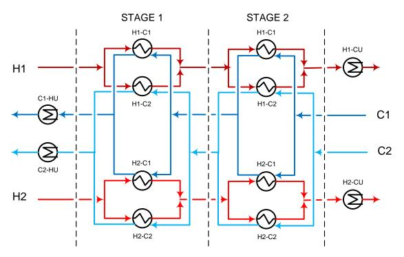
**Figure 7.5:** Superestructure for Synheat Model (Yee and Grossman, 1990) exemplified for two hot streams, to cold streams and two stages.
