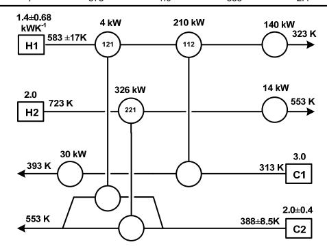
Figure 7.18: Flexible configuration for example 2.
