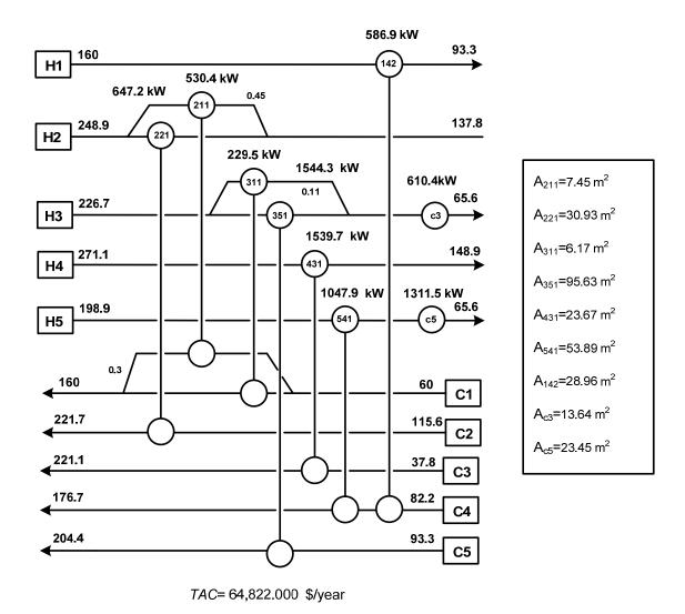
**Figure 4.6:** Heat Exchanger Network for Example 3 NLP improvement.
