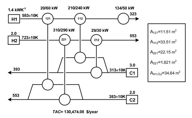
Figure 7.11: Final Configuration for Case Study 1.
