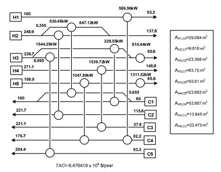
Figure 3A.5: HEN Configuration for the Case Study 02 using Synheat.
