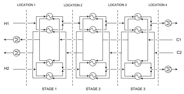
**Figure 3.9:** Simplified stage-wise Superstructure for HENs synthesis approach.
