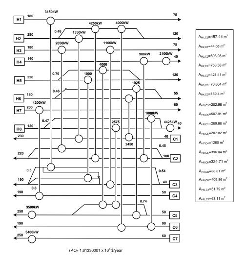
**Figure 3A.6:** HEN Configuration for the Case Study 03 using Superstructure.
