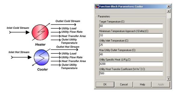
**Figure A.6:** Utility exchanger blocks, and configuration window for cooler block.
