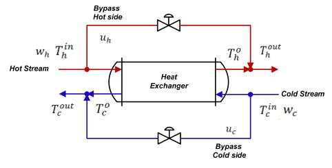
**Figure A.2:** General structure of a heat exchanger with bypasses.
