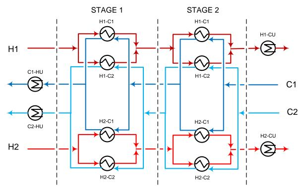
**Figure 6.2:** Two-stage Superstructure for two hot and two cold streams.
