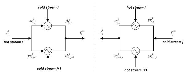
Figure 3.10: Illustration of the new variables needed for not assuming isothermal mixing.
