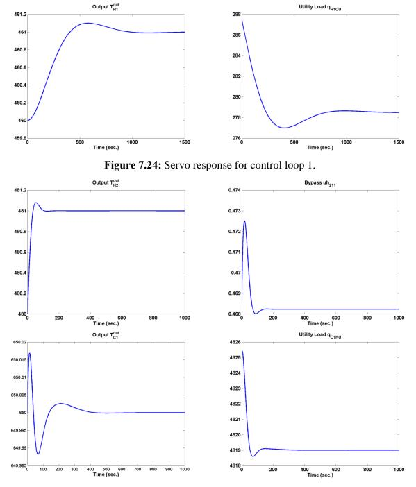
**Figure 7.25:** Servo response for control loop 2 and effect on control loop 7.
