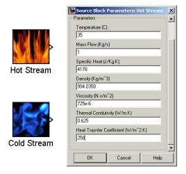
Figure A.4: Configuration window of the block stream.
