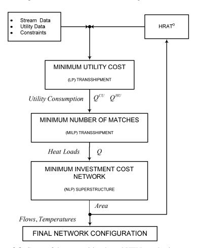
**Figure 3.8:** Steps of decomposition based HEN synthesis approach.
