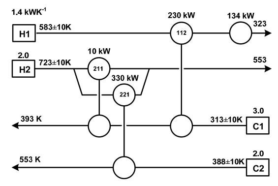
**Figure 6.3:** Heat Exchanger Network for Example 1.
