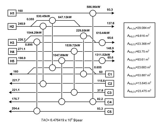
Figure 3A.4: HEN Configuration for the Case Study 02 using Hyperstructure.
