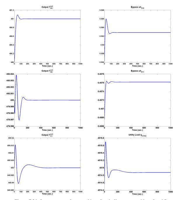
**Figure 7.26:** Servo response for control loop 3 and effect on control loop 2 and 7.
