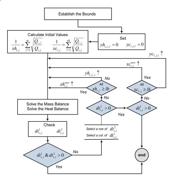
**Figure 3.12:** NLP initialization procedure for a feasible starting point.
