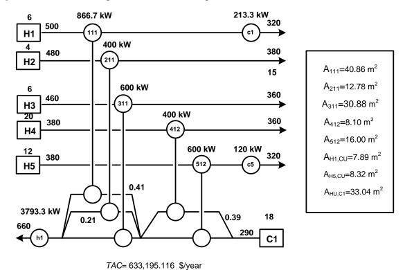
**Figure 4.4:** Heat Exchanger Network for Example 2 with NLP improvement.
