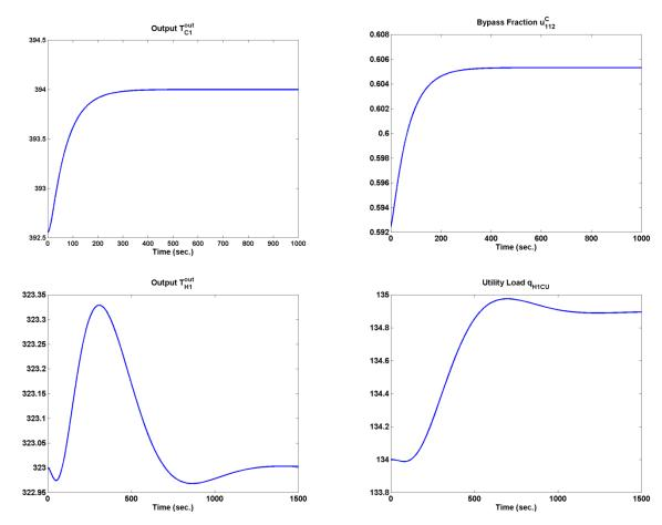
Figure 7.15: Servo response for control loop 3, and effect on loop 1.
