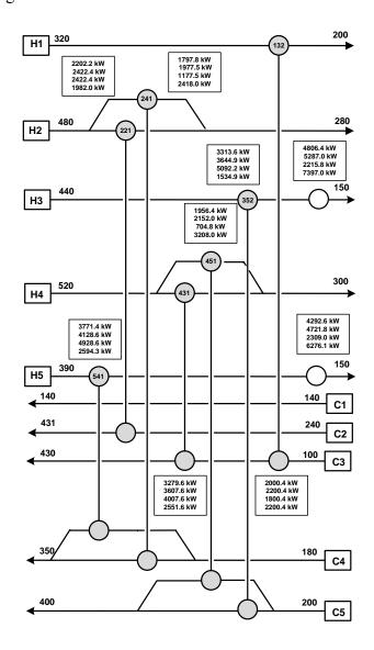
**Figure 5.7:** Multiperiod Synthesis for periods 1,2,3, and 4 for example 2.
