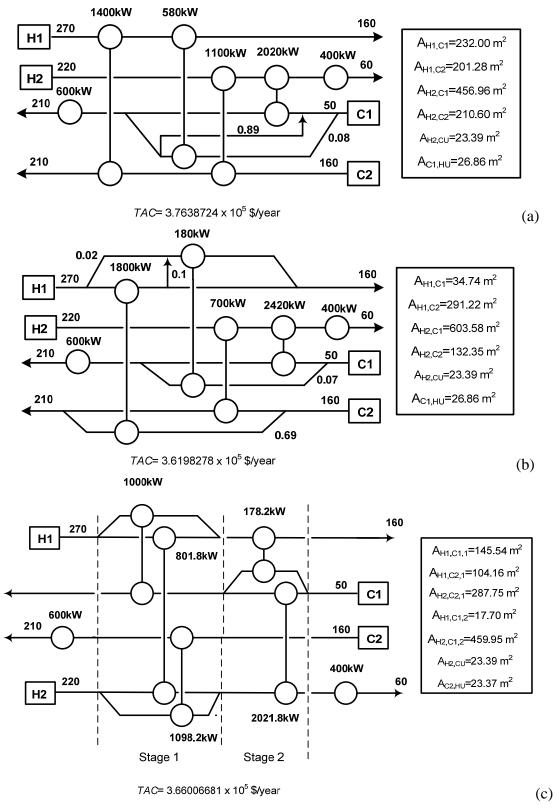
**Figure 3A.2:** HEN configuration for Case Study 01 using Superstructure (a), Hyperstructure (b) and Synheat Model (c).
