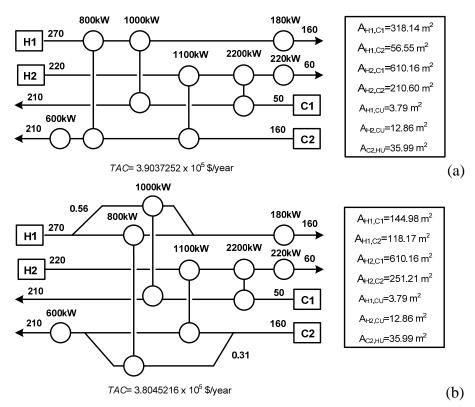
**Figure 3A.1:** HEN configuration for Case Study 01 using Pinch Technology (a), using NLP Superstructure using Pinch Solution as initial point (b).
