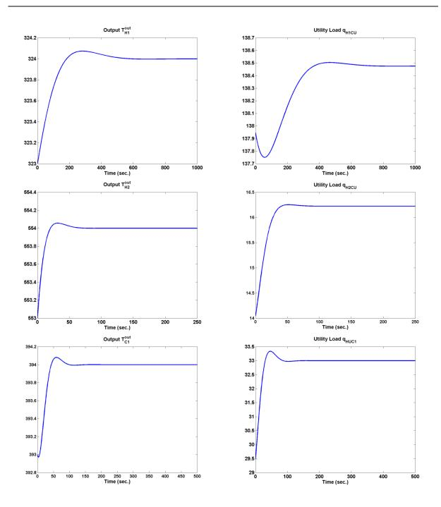
Figure 7.20: Servo response for the loops controlled by utility loads.
