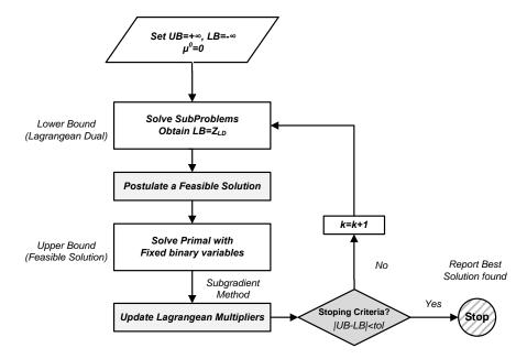
**Figure 5.4:** Lagrangean Heuristic Approach for solving multiperiod Synheat model.
