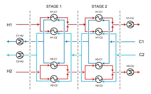
**Figure 5.3:** Superestructure for Synheat Model (Yee and Grossman, 1990) exemplified for two hot streams, to cold streams and two stages.
