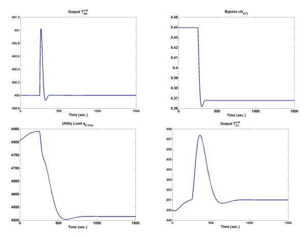
**Figure 7.29:** Regulatory response for all control loops, from nominal conditions to critical point 2 at 250 seconds.
