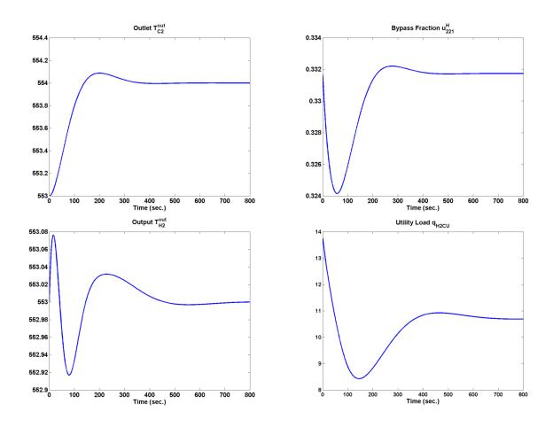
Figure 7.21: Servo response for control loop 4 and effect on control loop 2.
