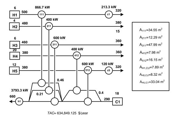
**Figure 4.3:** Heat Exchanger Network for Example 2 from the MINLP solution.
