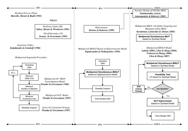
**Figure 5.2:** General Overview on methods for Design of Flexible HENs.
