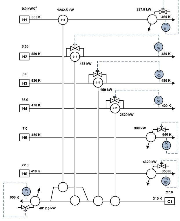
**Figure 7.23:** Final configuration and control structure for the example 3.
