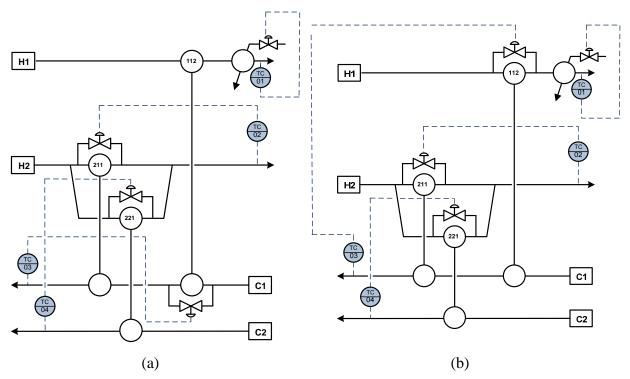
Figure 7.10: Two possible Control Structures for Nominal Design.
