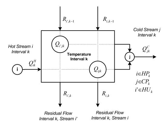
**Figure 3.6:** Graphical representation of temperature interval k for the MILP transshipment model.
