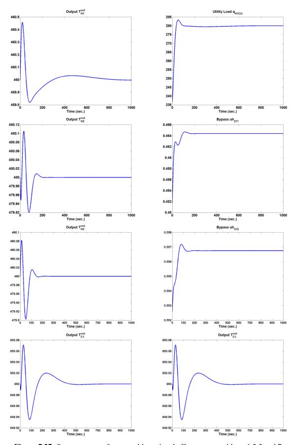
**Figure 7.27:** Servo response for control loop 4 and effect on control loop 1,2,3 and 7.
