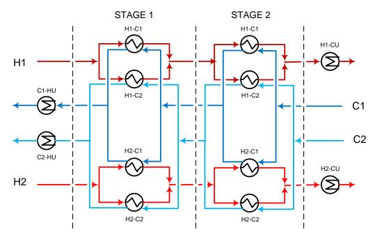
**Figure 4.1:** Two-stage Superstructure for two hot and two cold streams.
