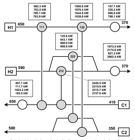
**Figure 5.6:** Multiperiod synthesis for Example 1 and periods, 1,2,3, and 4...
