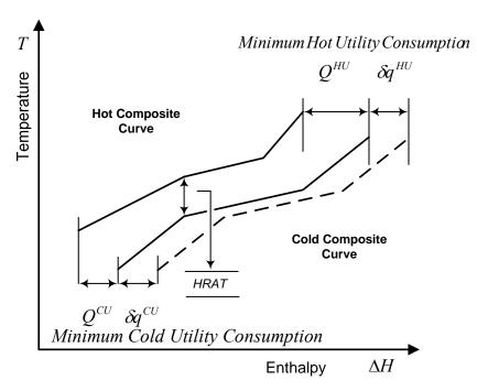
Figure 3.3: Composite curves and Pinch illustration.
