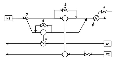
Figure 7.2: Possible manipulated inputs in HENs.
