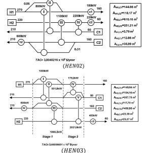
**Fig. 2.** HENs Designed for the Case Study u for  $\Delta T_{min} = 10$ using different approaches.
