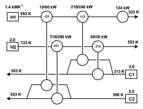
**Figure 6.4:** Heat Exchanger Network for Example 1 at iteration 2.
