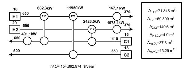
**Figure 4.2:** Heat Exchanger Network for Example 1.
