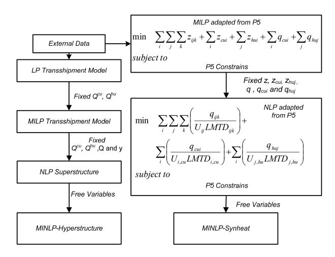
Figure 3.13: MINLPs initialization procedure for a feasible starting point.
