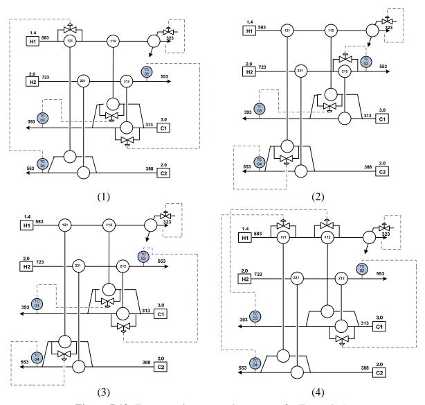
**Figure 7.12:** Four promising control structures for Example 1.
