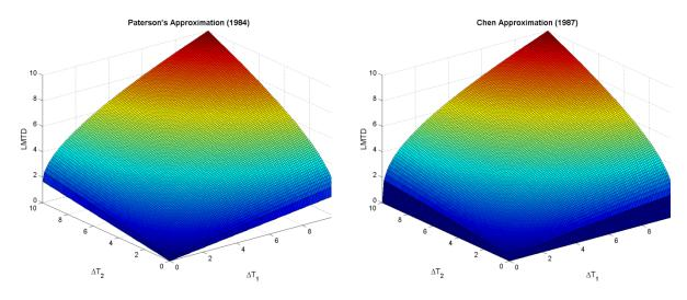
Figure 3.16: Log mean temperature approach approximations.
