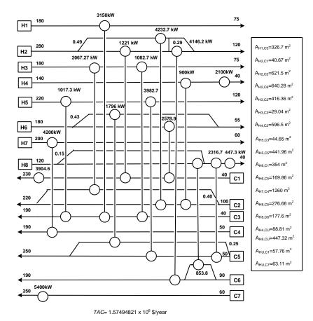
**Figure 3A.7:** HEN Configuration for the Case Study 03 using Hyperstructure.
