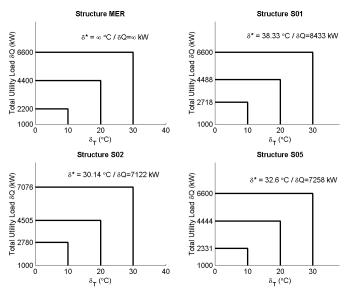
Fig. 6. Total utility consumptions at the critical operating conditions versus the flexibility ranges for structures MER, S01, S02 and S05.
