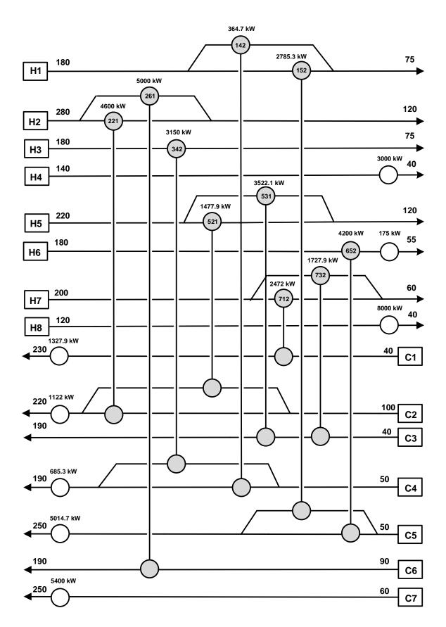
**Figure 5.8:** Multiperiod Synthesis for periods 1,2,3, and 4 and example 3.
