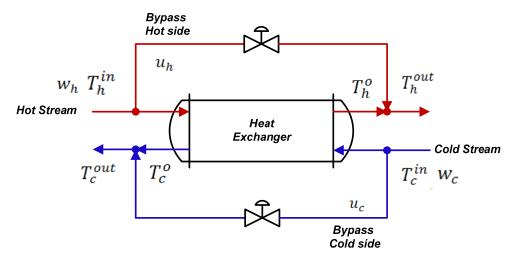
**Figure 7.6:** General heat exchanger with bypasses.
