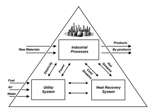
**Figure 7.1:** An overall process system.
