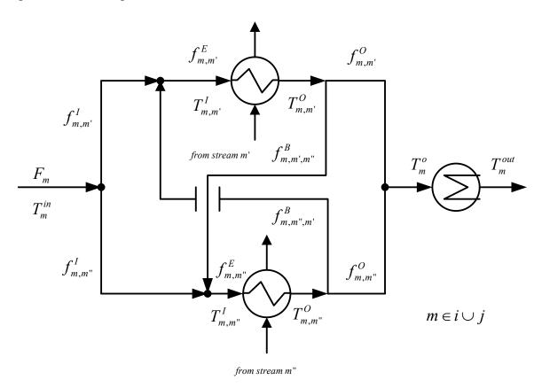
**Figure 3.7:** Graphical representation of the Network Superstructure.
