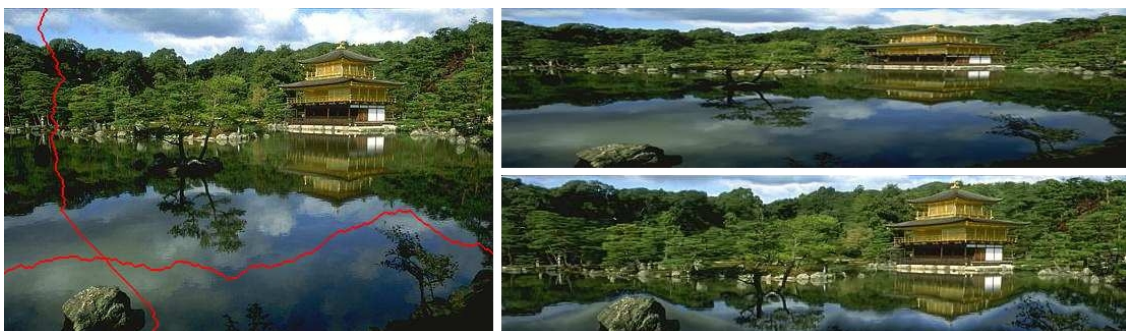
Figure 9.4: An example of image retargeting using the seam carving technique from Avidan and Shamir (AVIDAN; SHAMIR, 2007). The original image (left) resized using a traditional approach (top-right) and using the seam carving method (bottom-right). The red paths of the input image are examples of seams. Source: (AVIDAN; SHAMIR, 2007).
