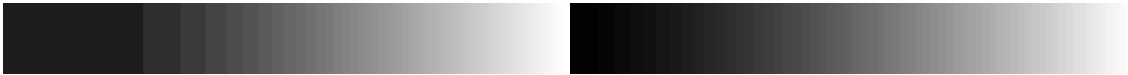
Figure 2.7: A linear encoding (left) takes fixed steps to quantize luminances. Since luminances are perceived non-linearly, in a logarithm fashion, abrupt changes are more noticeable in darker regions. A gamma encoding (right) uses a variable step size for quantization, providing a better fitting for the logarithm nature of the HVS responses to luminances. A good encoding keeps the relative difference of two close quantized intensities below the visible threshold of 1%. Source: (WARD, 2005).
