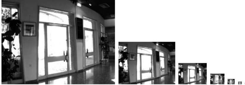
Figure 7.6: The mip-map levels of the relative luminance image L_r . The single texel of the last mip-map level is the average \overline{L_r} of the entire relative luminance image.
