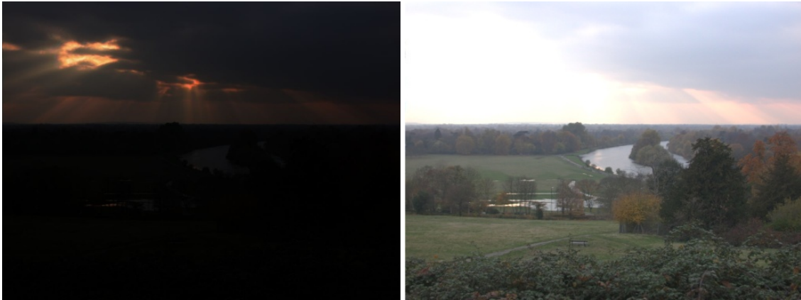
Figure 2.6: Automatic luminance compression using a linear scaling (left) and a gamma compression (right). The former loses almost all of the details of the image. A gamma compression is more attractive, but it still is far away from the results expected from Figure 2.4.
