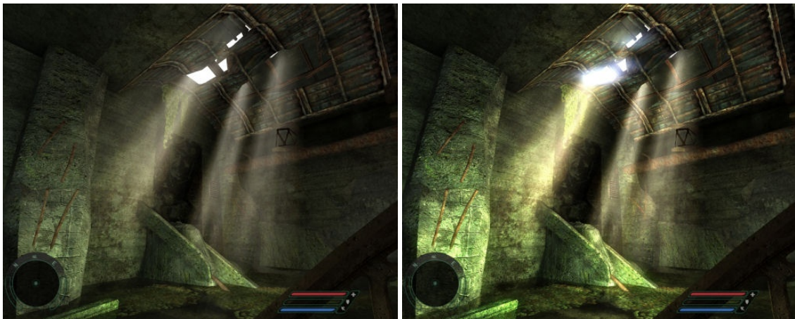
Figure C.4: Two screenshots from the game FarCry: the image on the left does not use HDR rendering, while the one on the right performs, using a tone-mapping operator to compress the dynamic range of the image. Source: Wikipedia.
