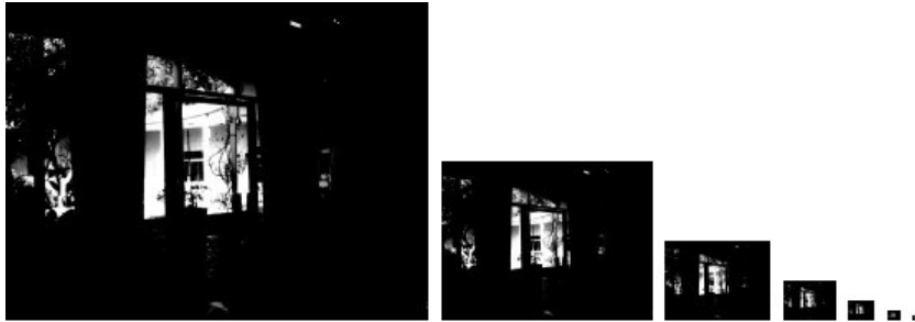
Figure 7.4: The mip-map levels of the log-luminance image L_{log} . The single texel of the last mip-map level is the averaged sum of Equation 4.5, but still without the exponential function.
