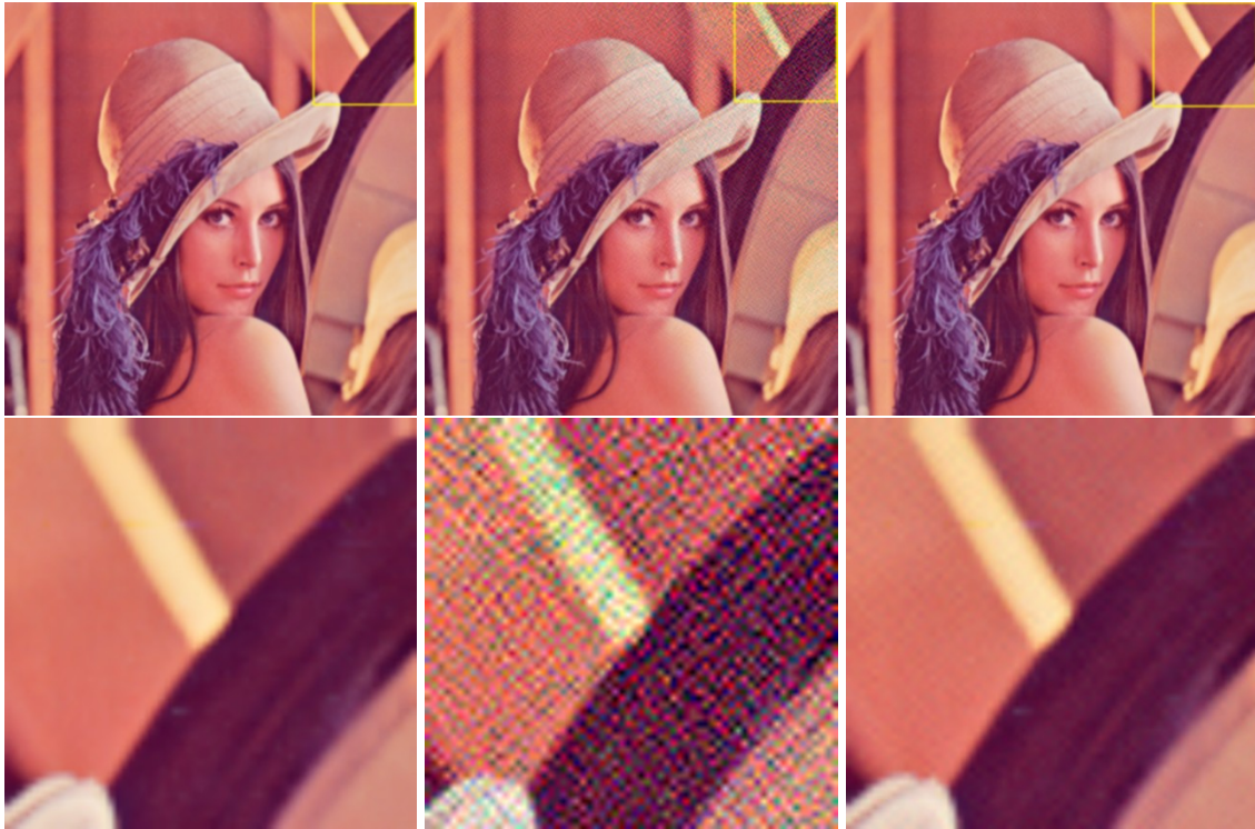
Figure 5.17: Example of precision loss on summed-area tables. In the first column, the original table (image). The middle column is a reconstruction of the original image using its corresponding summed-area table. The last column is an improved reconstruction that minimizes the precision loss. Bottom images are zoomed versions of the top images. All SATs were built using 24-bit floats. Note that the artifacts appear in the top-right portion of the image, instead of the bottom-right. This is because, in OpenGL, textures are parametrized from left to right and bottom to up, so the resulting SAT is flipped vertically. Source: (HENSLEY et al., 2005).
