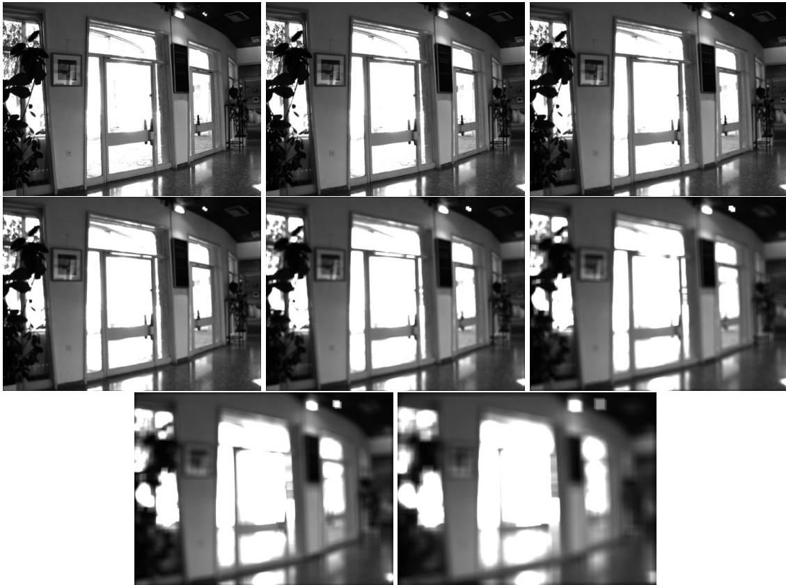
Figure 7.8: The relative luminance image filtered at different scales (adaptation zones), obtained using box-filtering (Equation 7.1). The kernel sizes are the same from Figure 7.8.
