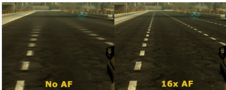
Figure 2.6: Comparison of a game scene without anisotropic filtering and with anisotropic filtering with 16 samples. Notice how the white stripes in the road become blurry as they get distant from the viewer when anisotropic filtering is off.
