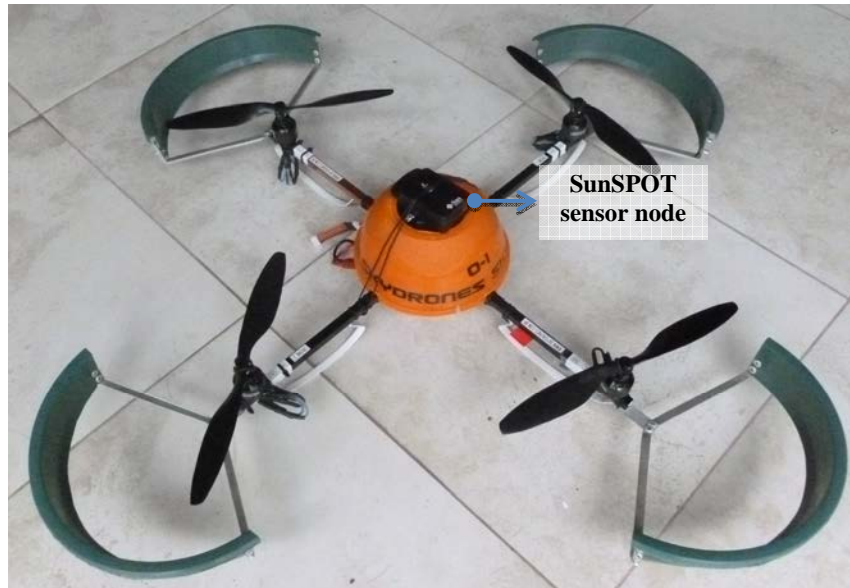
Figure 7.5: SunSPOT sensor node mounted on top of the quadcopter platform.
