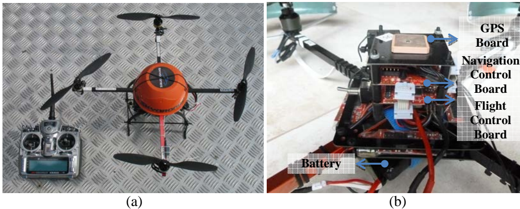
Figure 7.4: Quadcopter platform: a) quadcopter and remote control; b) internal electronic devices.
