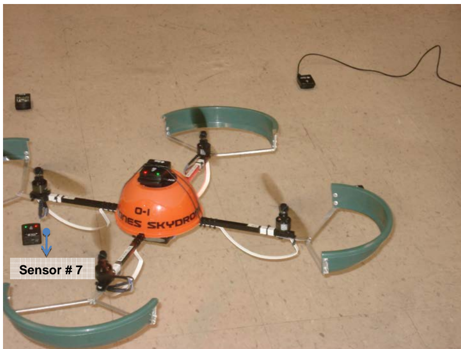
Figure 7.15: Third step of the test – after the alarm is issued, it is correctly delivered by the static sensor node that is closer to the mobile sensor node (the one that has the highest pheromone level).
