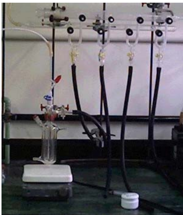
Figure 21. Double walled glass reactor (120 mL) used for Tandem synthesis of LLDPE.
