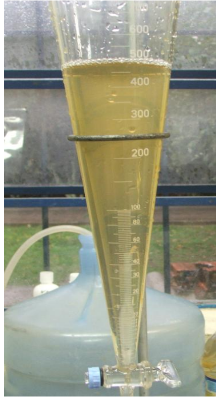
Figura 11. DAM no Cone de Imhoff.
