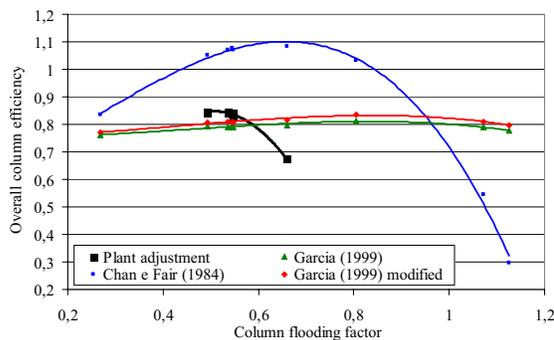
**Fig. 3.** Comparison of overall efficiency of the C6 column (valve tray) with the efficiency prediction models.
