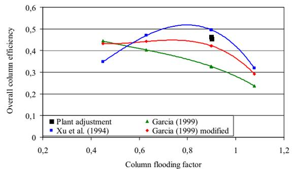
**Fig. 4.** Comparison of overall efficiency of the Propylene column (dualflow) with the efficiency prediction models.
