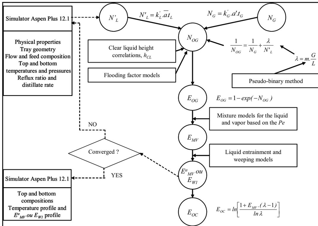
Fig. 2. Algorithm used in the Aspen Plus 12.1 simulator for the calculation of Murphree apparent tray efficiency ( $E_{MV}$  or  $E_{WI}$ ).
