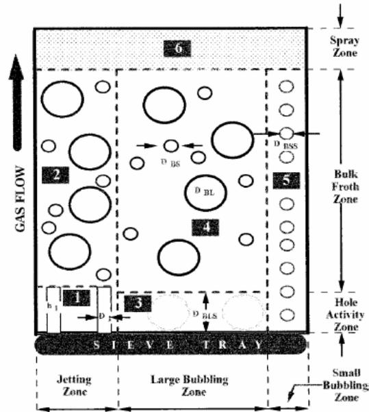
Fig. 1. Hydraulic dispersion model above the tray (Prado and Fair, 1990).
