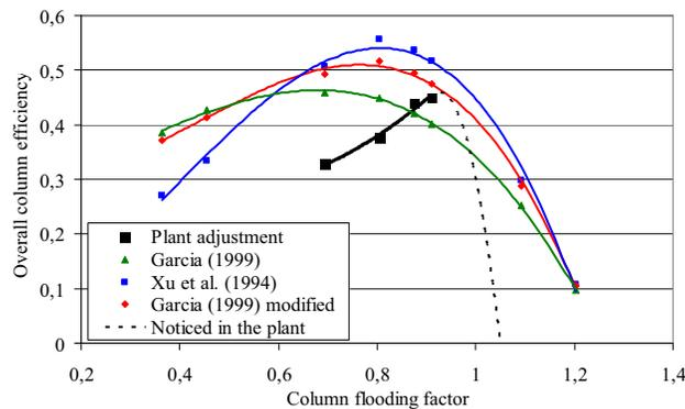
**Fig. 5.** Comparison of overall efficiency of the Butene-1 column (dualflow) with the efficiency prediction models.
