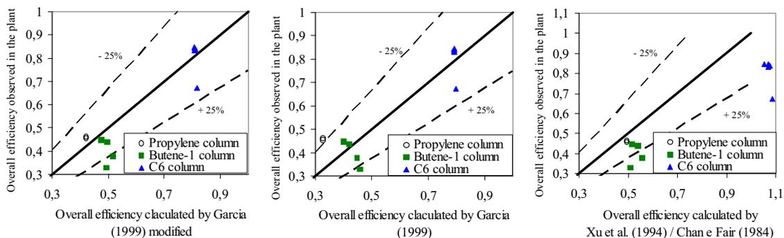
**Fig. 6.** Comparison between overall efficiency calculated by Garcia (1999) – modified, by Garcia (1999) original and by Chan e Fair (1984) and Xu et al. (1994), respectively values observed in industrial columns.
