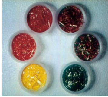
Figure B.14: Color sequence of a continuous series formed by crystals of CdS and CdSe (SHEVELL, 2003).
