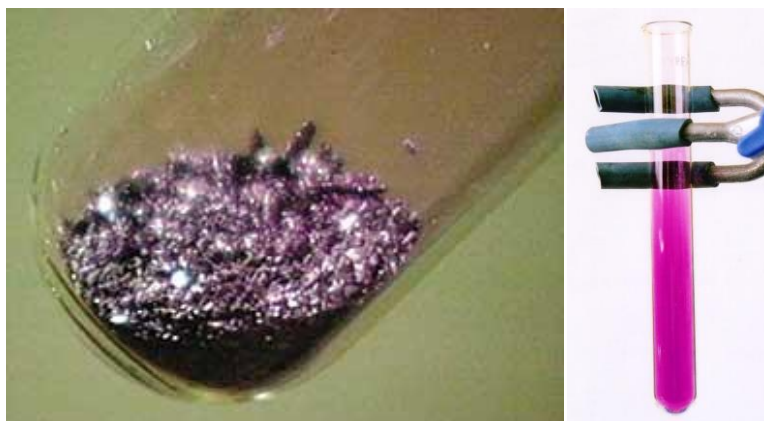
Figure B.6: Iodine in solid state (left), and vaporized (right) (Disponível em: https://www.chem.wisc.edu/deptfiles/genchem/lab/ptl/Elements/i/I.html . Acesso em: Jun. 2012)
