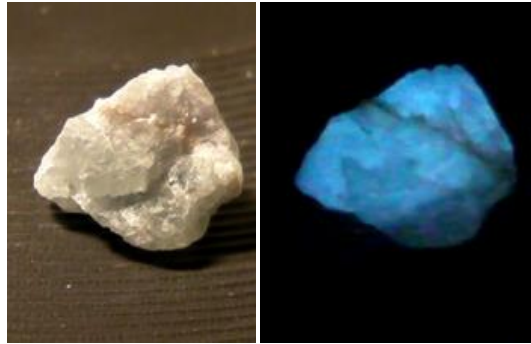
Figure 2.16: Thermoluminescence in fluorite before (left) and after heating (right) (Disponível em: http://en.wikipedia.org/wiki/Thermoluminescence . Acesso em: Jun. 2012).
