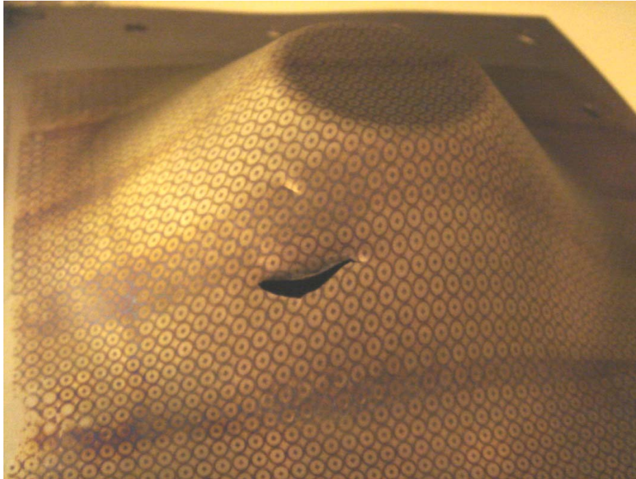
Figure 31: Fracture of the material presented in SPIF of cone with angle of 45°.
