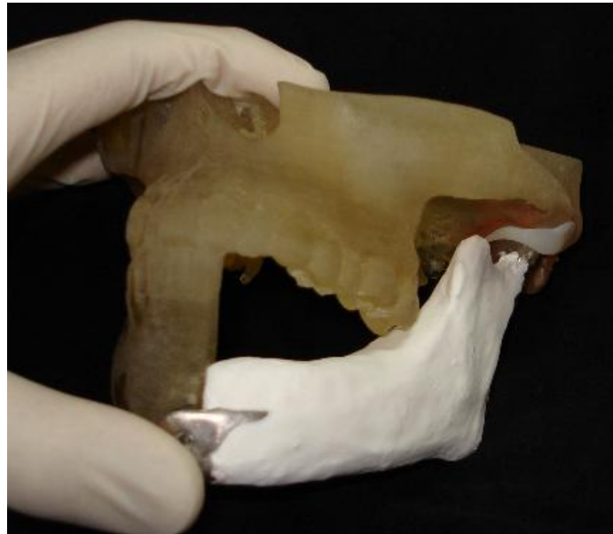
Figure 3: Physical biomodel, produced through additive manufacturing and used to the project of a mandibular prosthesis.
