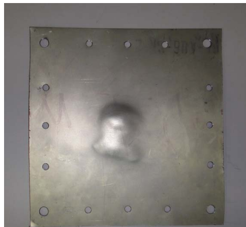
Figure 41: Incremental forming of implant for repair of cranial defect.
