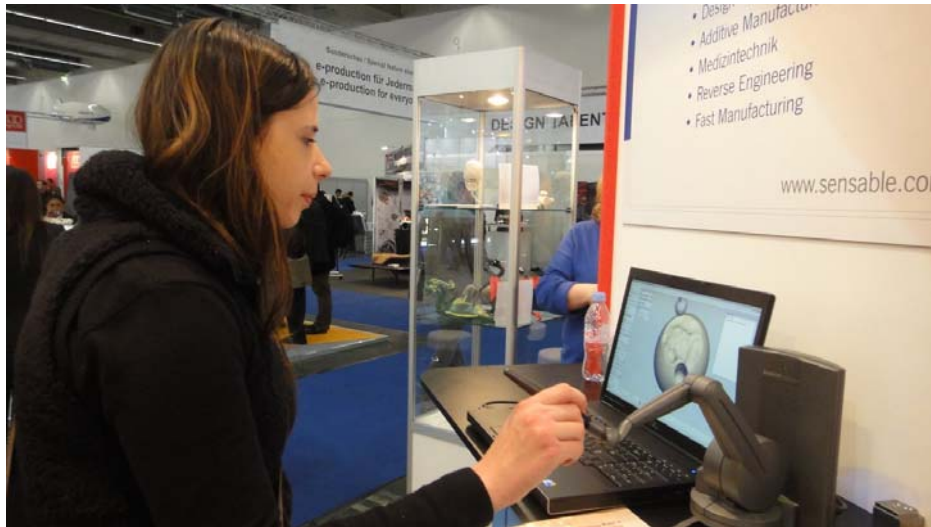
Figure 8: Phantom Omni haptic device, from the company SensAble, which causes a tactile feedback to the user.
