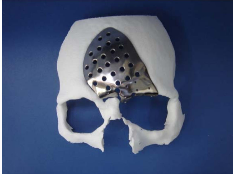
Figure 44: Resulting cranial implant produced through manual shaping.
