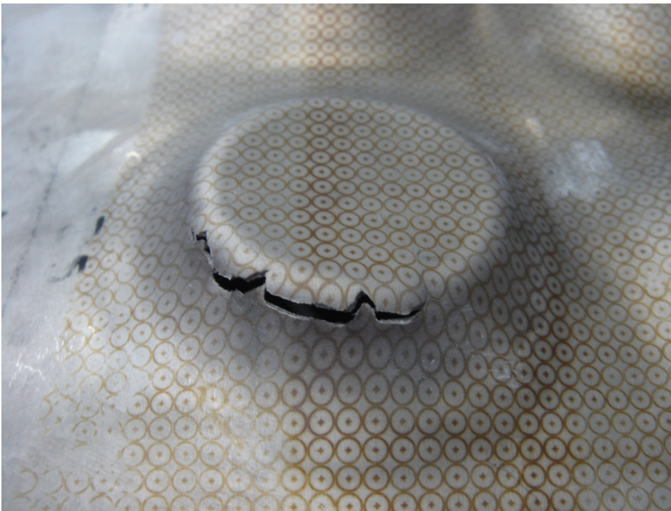
Figure 30: SPIF in titanium cone forming an angle of 50° with the plane of the plate, with disruption.
