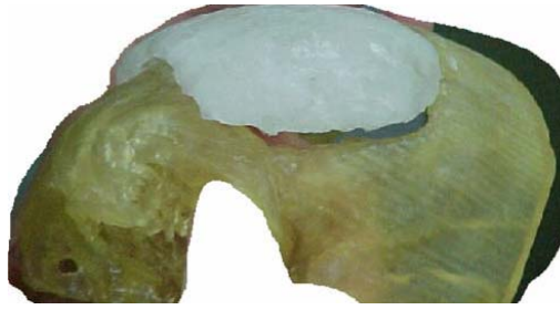
Figure 7: Prototype of the cranial implant manually modeled in wax. Source: Maji et al. (2008).
