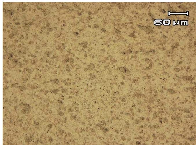
Figure 26: Metallographic analysis of titanium samples, showing equiaxed microstructure.
