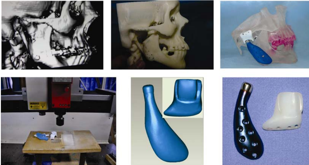
Figure 17: Manufacture of custom TMJ prosthesis. a) CT scan of the patient. b) Anatomical biomodel showing the removal of region to be replaced. c) Prosthesis prototype. d) Scanning of the components of the prototype. e) Virtual model. f) Final prosthesis, manufactured through CNC milling.
