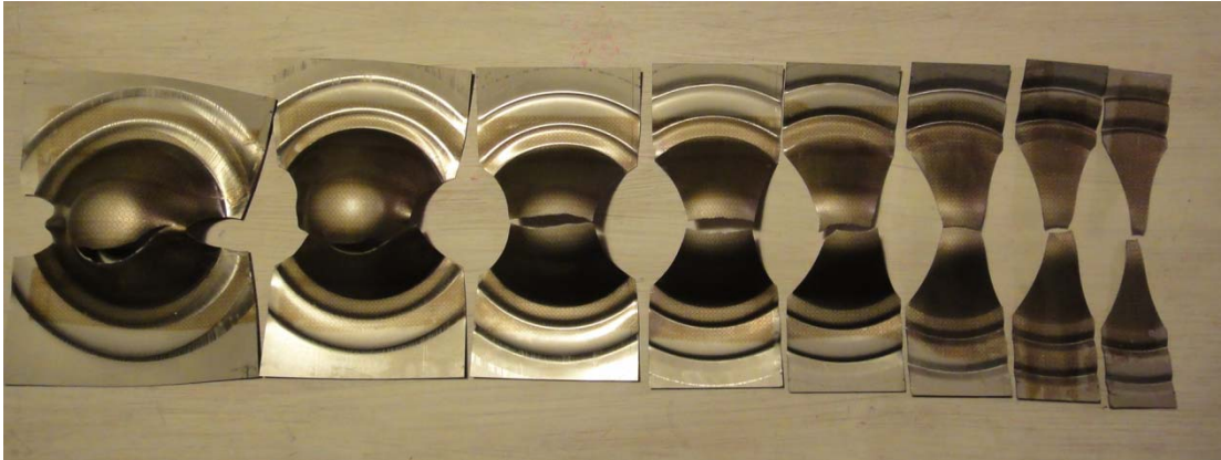
Figure 20: Testing specimens submitted to a forming test to determine the Forming Limit Curve of the material.
