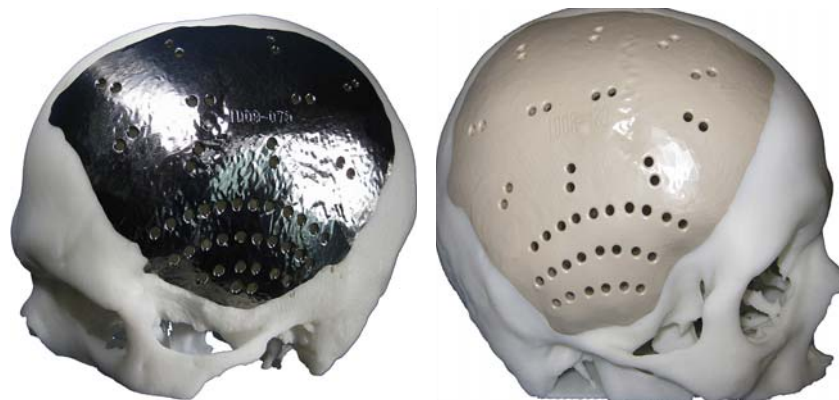
Figure 11: Custom prosthesis for reconstruction of cranial defects, modeled in CAD and manufactured through CNC machining.
