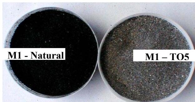
FIGURA 4.33 Mistura M1 tratada com TQ5 ( $\text{HCl} + \text{H}_2\text{SO}_4$ )
