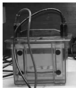
Sistema vertical Slab Gel BIO-RAD Mini-Protean II (BioRad Laboratories, Richmond, CA, USA)
