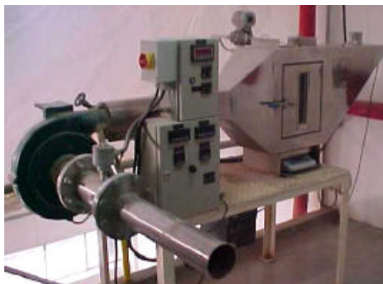
Fig. 1. Pilot dryer used in the determination of the drying curves.
