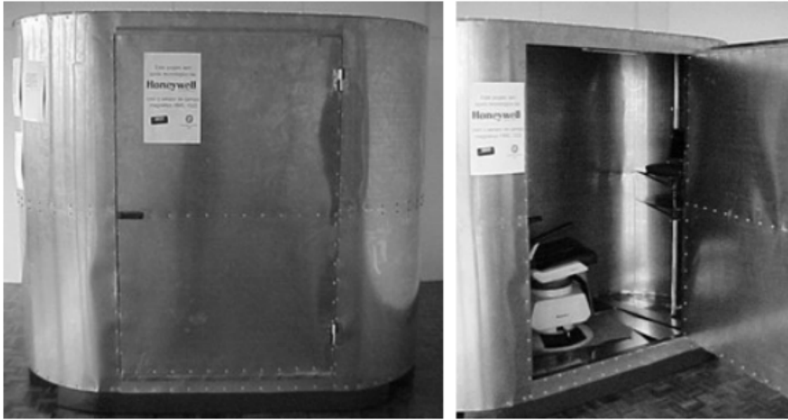
Figure 3.7: The ambient where the EEG measurements were performed, following the concept of a Faraday Cage.
